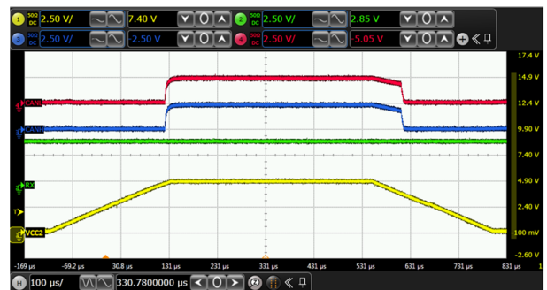
Figure 6-14. Glitch Free Power Up on V_{CC2} – CAN Bus Remains Recessive
