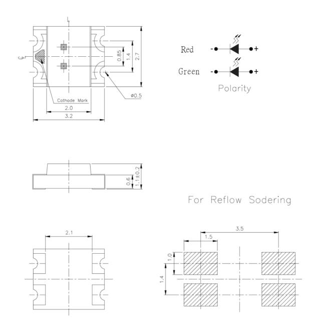
**Note:** The tolerances unless mentioned is  $\pm 0.1 \text{ mm}$ , Unit = mm
