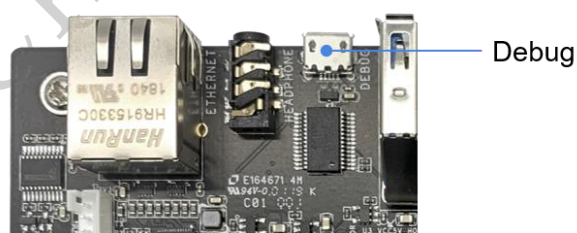
Fig 2-4 USB Uart Debug interface
