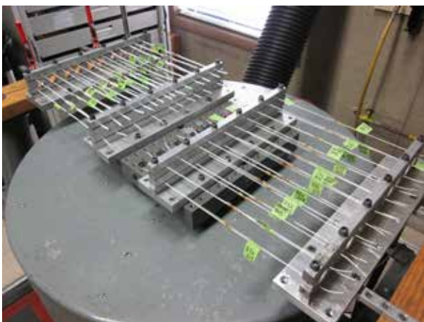
Figure 2 - Military Vibration Test - SOLISTRAND Splices
