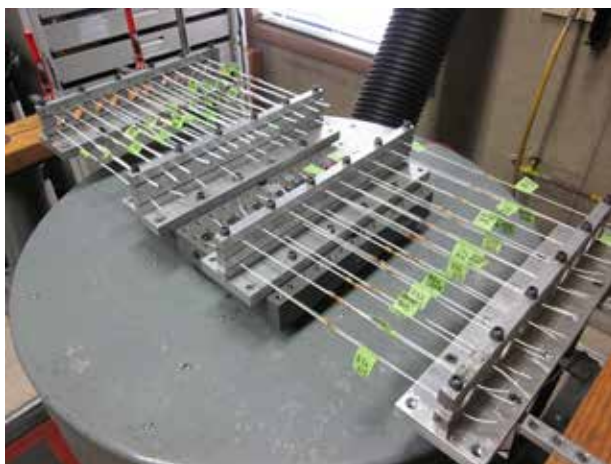
Figure 2 - Military Vibration Test - SOLISTRAND Splices
