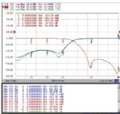
2012 / 3.5GHz Wimax Low Pass Filter CFL4111714503504K
