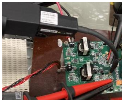
(b) Measurement using an optical isolation probe
