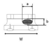
External appearance criterion for exposed wire Exposed end of the winding wire at the secondary side should be 2mm and below.
