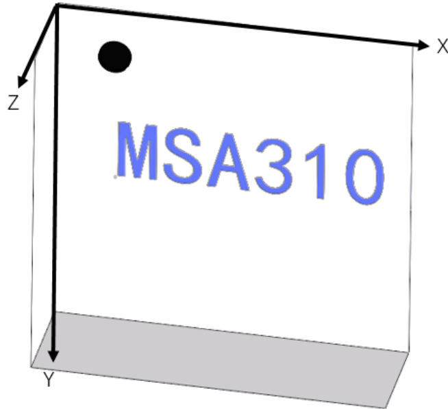
Figure 10: Orientation of sensing axis
