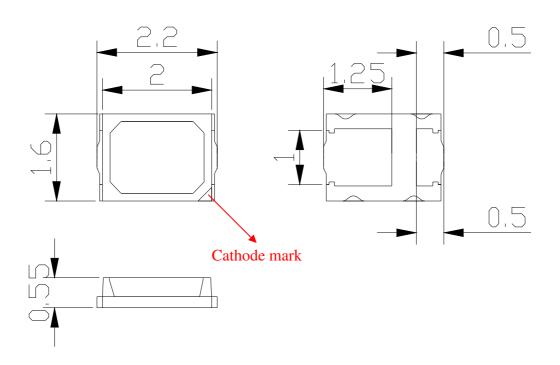
Unit: mm, Tolerance: ±0.1mm
