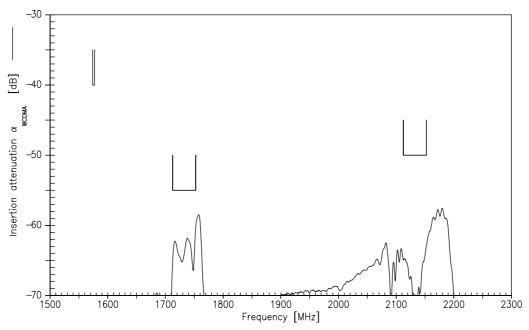
Power Transfer Function Tx-Rx isolation (Wideband):
