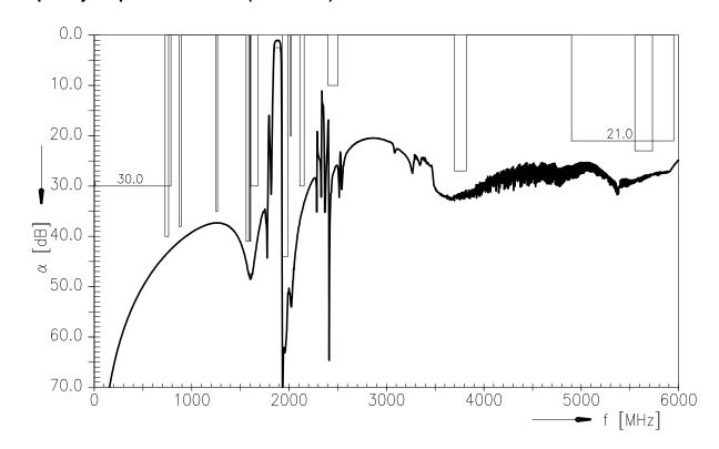
Frequency response ANT - RX (passband, averaged value of linear s-parameter over 5 MHz)
