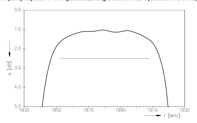
Frequency response TX - ANT (averaged value of linear s-parameter over 5 MHz)
