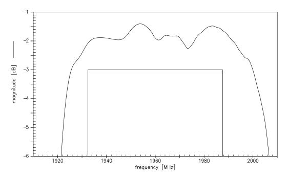
Transfer function for WCDMA signals (Power transfer function narrowband)
