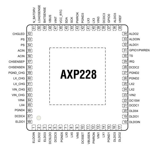
Figure 2. AXP288 Pin Configuration
