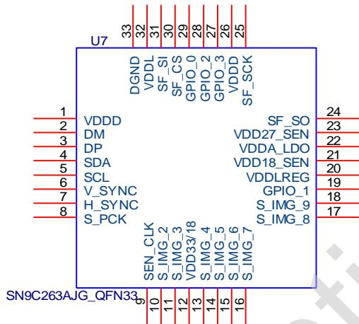
\*\*Pin33 is the package bottom pad of IC,
