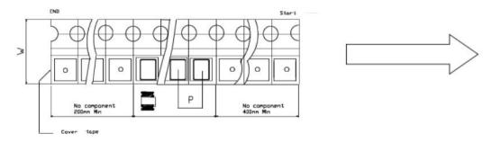
Note: After the tape is woven, the outermost layer of the reel is 400mmMIN, and the innermost layer is 200mmMIN.
