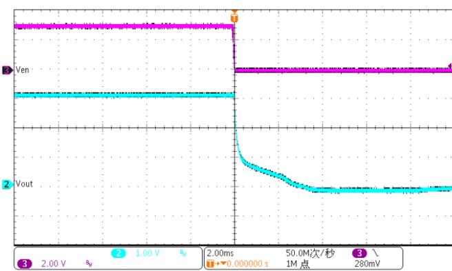
Turned off from EN @No Load , V<sub>IN</sub>=3V
