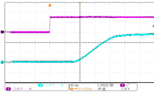
Turned on from EN @No Load , V<sub>IN</sub>=3V
