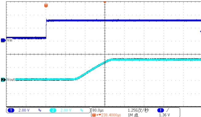
Power on from V<sub>IN</sub> @No load, V<sub>EN</sub>=3V
