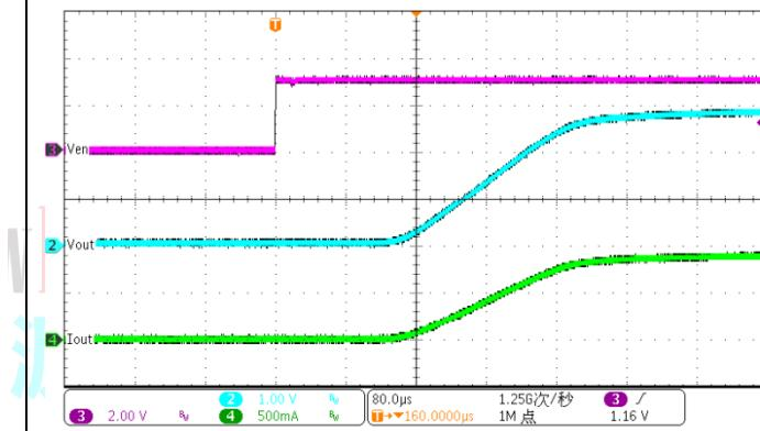
Turned on from EN @ Load=3R, V<sub>IN</sub>=3V
