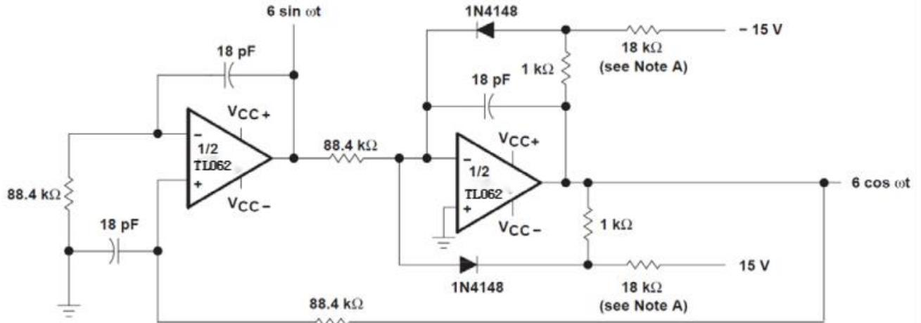
NOTE A: These resistor values may be adjusted for a symmetrical output.
