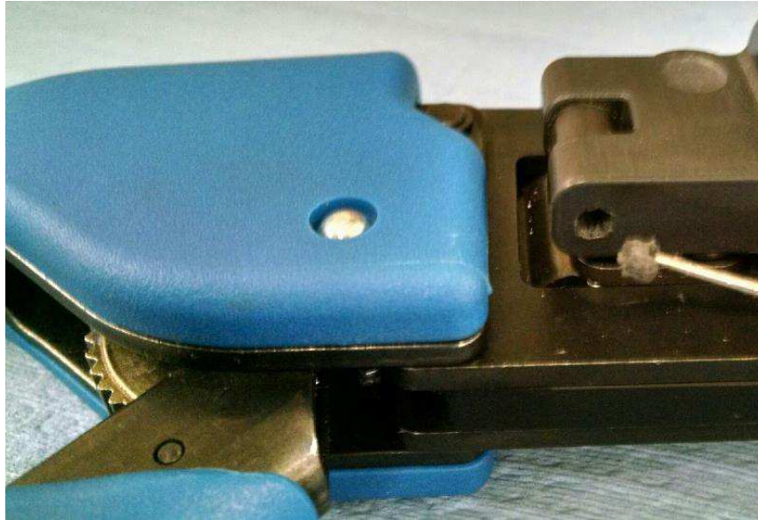
Figure 3: Removing RTV sealant
