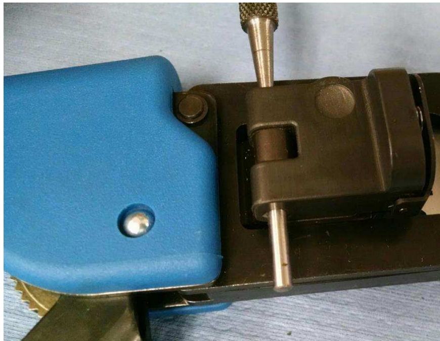
Figure 4: Removing dowel pin
