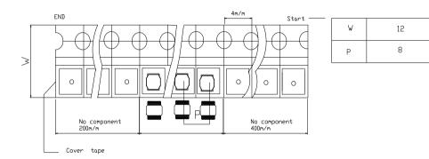
Note: After the tape is woven, the outermost layer of the reel is 400mmMIN, and the innermost layer is 200mmMIN.
