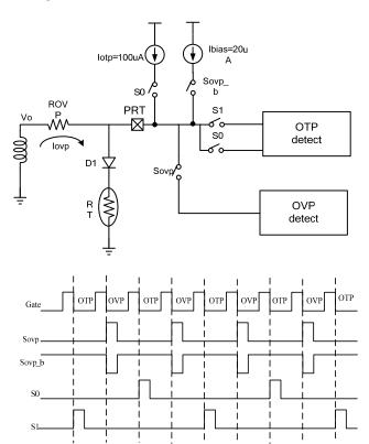
On-Bright proprietary dual function of external OTP and output OVP provides feasible and accurate detection of external OTP through NTC resistor and output OVP. The dual function is
