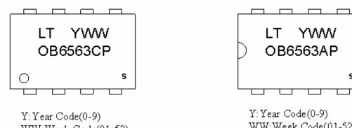
WW: Week Code(01-52) C:SOP8 Package P:Pb-free Package S:Internal Code(Optional)
