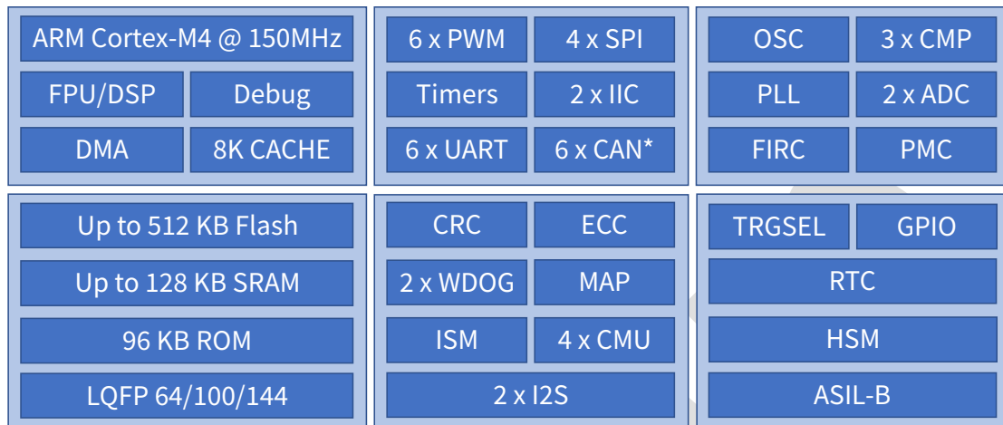
Figure 2. FC4150F512 block diagram
