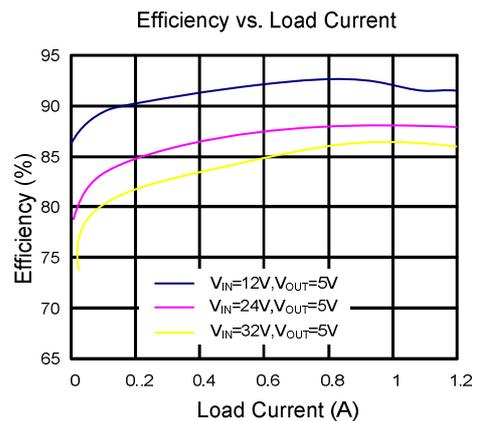
Figure 2. Efficiency Figure
