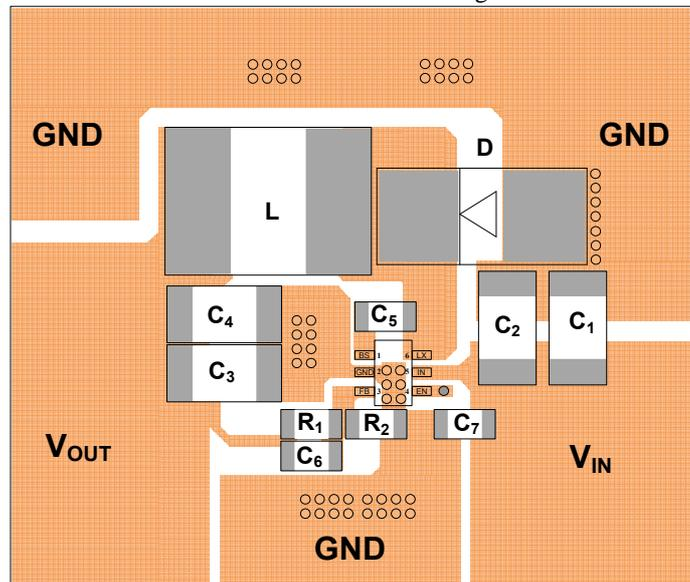
The layout design of SY8291 regulator is relatively simple. For the best efficiency and minimum noise problem, we should place the following components close to the IC:  $C_{IN}$ , L, R1 and R2.
