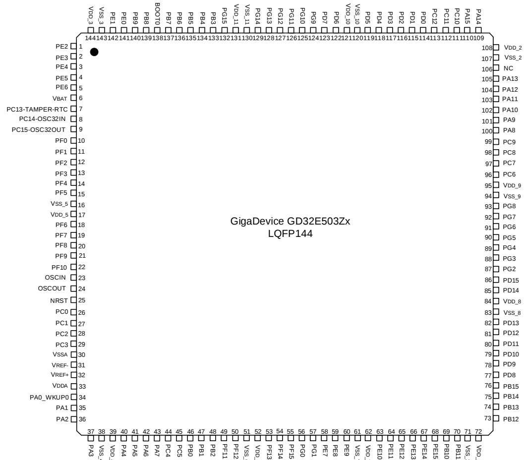
Figure 2-2. GD32E503Zx LQFP144 pinouts
